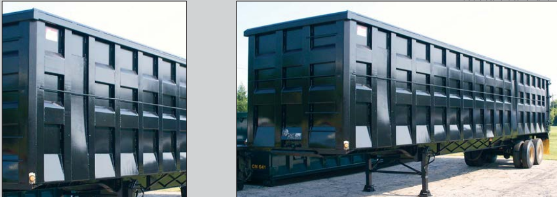
Extra heavy duty trailer with two (2) rows of deltas and two (2) vertical stiffeners
